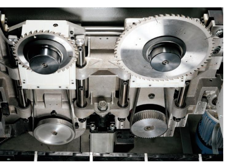
The superior cutting quality is achieved through independent rise and fall movements of the main blade and the scoring blade.
