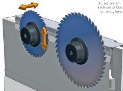
Fast, accurate setting of the scoring and main blades, using Digiset system. The system also stores the information for each set of blades, ensuring repeatable and accurate alignment every time.
