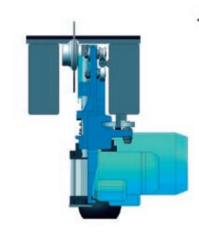
The blade is not subject to any vibration, thanks to the upper guide, positioned next to the blade-holder spindle.
