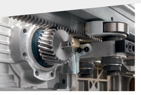
The perfectly linear movement of the tool holder carriage is achieved through a helical rack and pinion system and is driven by a brush-less servomotor.
