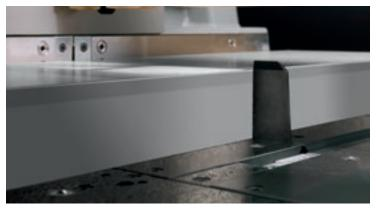
Perfect alignment of very thin and/or flexible panels, minimising cycle times thanks to the side alignment stop integrated in the blade carriage.
