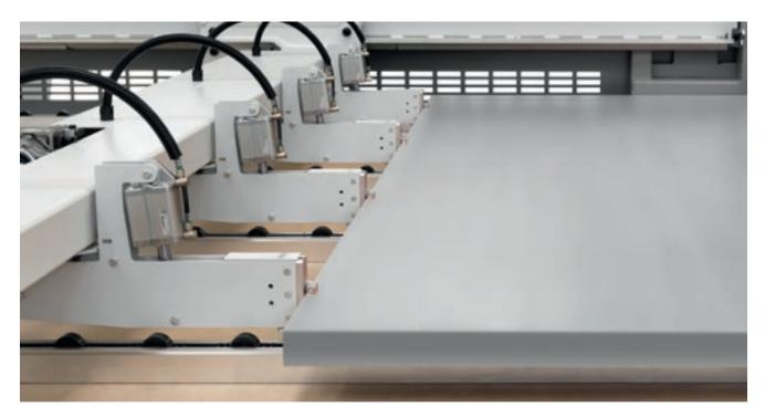
Fast, accurate positioning of the panels for optimum cutting precision, thanks to the robust pusher carriage activated by a brushless motor. The slide surface below the pushing device is fitted with independent rollers to avoid making any marks on panels with a delicate surface.
